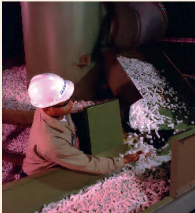
Latex is coagulated and then dried on a conveyor for use in the production of automobile and truck tires.
