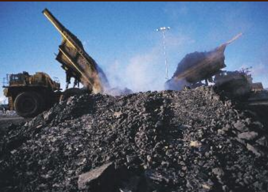
One of the world's largest resources of oil sands is located in Alberta, Canada. The sands are moved out to processing plants—at the rate of 500,000 tons per day—by the world's largest Caterpillar trucks.
