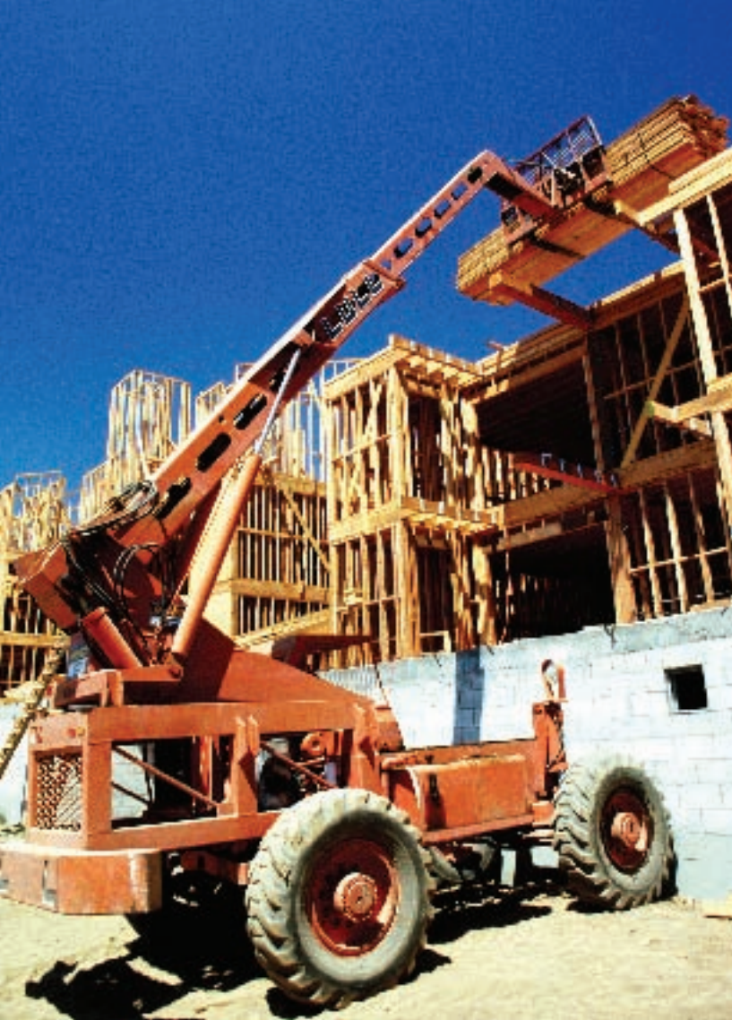
Tractors built with front-end loaders use a telescopic boom to extend their reach. They are often used to lift less cumbersome loads like lumber on this construction site in Los Angeles, Calif., left.
