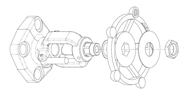
The lower thrust collar and yoke sleeve can now be removed from the bonnet.
