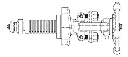
Turn the handwheel clockwise to push the stem out of the yoke sleeve. Once the stem is clear of the yoke sleeve, remove the stem from the bonnet. Remove the top gasket.
