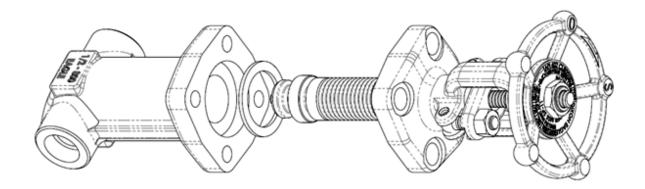
Loosen the gland nuts to loosen the packing.
