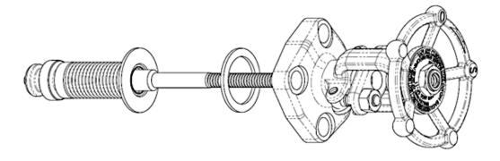
Remove the bellows assembly from the stem by unscrewing. Remove soft seat by removing screw, lock washer and flat washer.
