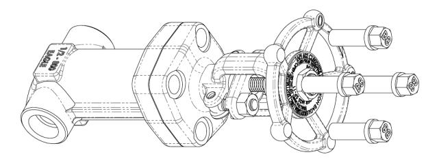
Lift the bonnet and stem assembly out from the body. Remove the lower gasket.
