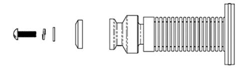
Remove the gland nuts fully. Take off the gland plate and gland bushing. Remove the packing from the bonnet. If replacing, unfasten the grease fitting and remove.
