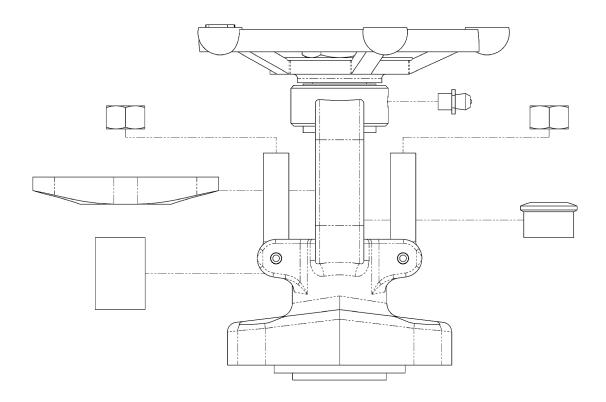
Unfasten the handwheel nut. Remove the nameplate, the handwheel, and the upper thrust collar.
